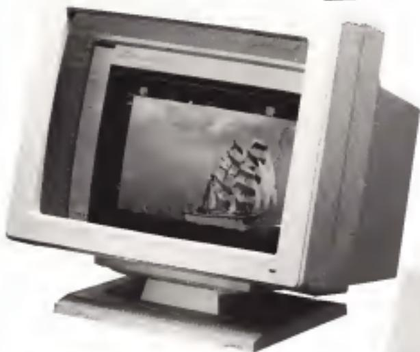
MONITOR AD ALTA RISOLUZIONE: 19" RGB ANALOGICO. SI ALLACCIA ALLE FREQUENZE TIPICHE DELLA VGA 640\*480 E DELLA VGA ULTRA 1024\*768. MEDIANTE SCHEDA 8514 O COMPATIBILE PUO' LAVORARE A 256 COLORI ANCHE NELLA RISOLUZIONE PIU' ELEVATA DI 1024\*768 CON I PIU' DIFFUSI PACCHETTI SOFTWARE GRAFICI. LA SCHEDA VGA 8514/A IBM COMPATIBILE, E' CIRCA 23 VOLTE PIU' VELOCE DI UNA NORMALE SCHEDA VGA E CIRCA 19 VOLTE PIU' VELOCE DI UNA SCHEDA 8514/A IBM.
